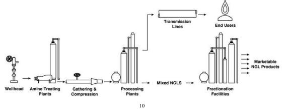
The following diagram illustrates the natural gas treating, gathering, processing, fractionation and transmission process.
