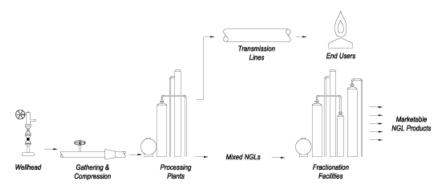
The midstream natural gas industry is the link between exploration and production of natural gas and the delivery of its components to end-user markets. The midstream industry is generally characterized by regional competition based on the proximity of gathering systems and processing plants to natural gas producing wells.
